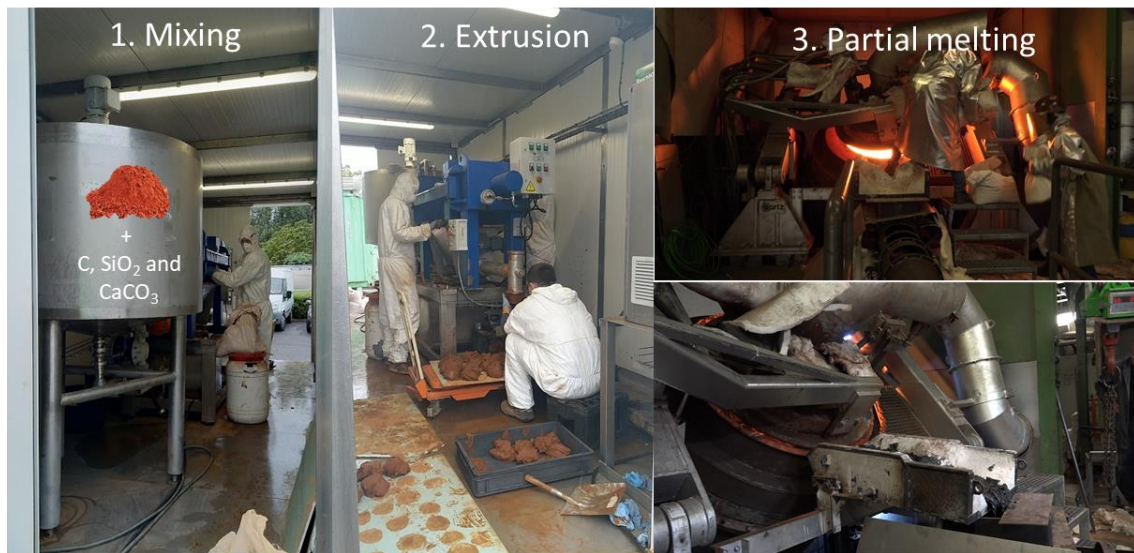
Figure 2: Steps of processing in the pilot plants in order to obtain VBR.
