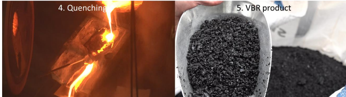
Figure 3: Left- Granulation of the partial melt; Right- The fine granulated material after quenching.
